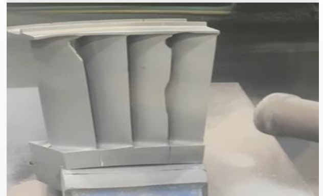
Damage to neighbouring blade
